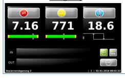
If the device is restarted, the dosing delay is running, during which time no dosing occurs.
