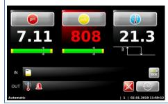
An alarm occurs; this is signalled by the symbol in the OUT list. The alarm relay is activated.
