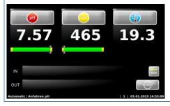
If one of the two measuring values, pH or mV, falls outside the control range, the start routine is activated.
