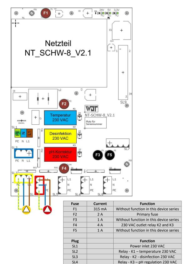
The picture shows an example of the connection of two external 230 volt dosing pumps (dosing devices).
