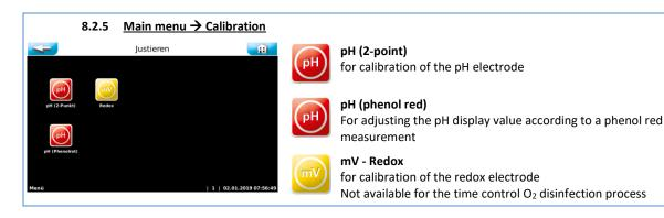
The calibrations are text-guided; the most important steps are explained in brief texts. Completed steps are acknowledged with the OK button. Values are adopted automatically once the measured electrode voltage remains stable for approx. 15 seconds.
