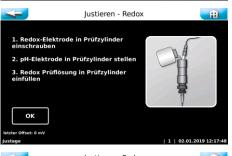
The Calibration → redox electrode menu enables a fine-tuning of the redox measurement. The redox test solution supplies a voltage of 468 mV at 25 °C, see bottle label.
