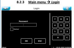
The controller can be protected by a password against unauthorised access. For rules for password assignment, see 8.2.1.8
