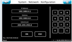
The control unit has a web front-end. The current measuring values and status reports can be transmitted to a home network via the network interface with an RJ45 socket. The terminal device can be a browser-enabled device such as a PC monitor, a tablet PC or a smartphone, e.g.
