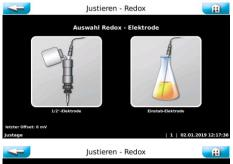
As a rule, the <code>IQntrol</code> DOS MODBUS device series is delivered with the  $\frac{1}{2}$ " redox electrode. Therefore, the menu on the left must be selected.
