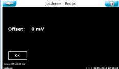
At the end of the menu, the set deviation is shown as Offset. In case of minor deviations, the calibration is adopted immediately.
